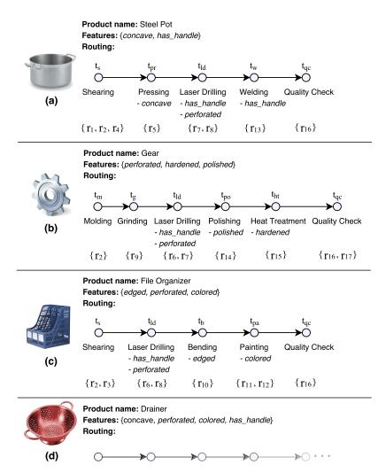
Fig. 2: The products being produced in the metal factory with their corresponding manufacturing processes: (a) Steel Pot with its process  $q_{sp}$ , (b) Gear with its process  $q_g$ , (c) File Organizer with its process  $q_{fo}$ , and the goal product (d) Drainer.
