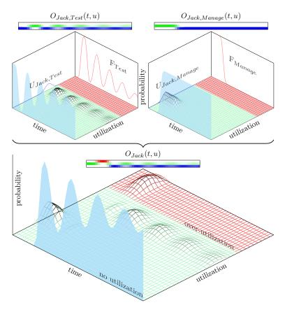
Fig. 5: Total Utilization PDF over time  $O_{\text{Jack}}$  of our running example and the relevant pieces it is composed of. Directly above the plots, we provide a more condensed visualization where the x-axis is time, and the y-axis is utilization. The color intensity is directly proportional with the probability density value. Note that the blue parts are of infinite slope caused by  $\delta(u)$ .
