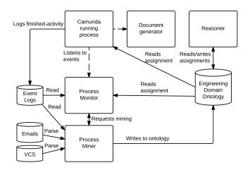
Fig. 9: Software architecture of the prototype
